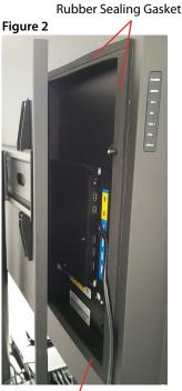
Route cables trough the bottom of the door only
